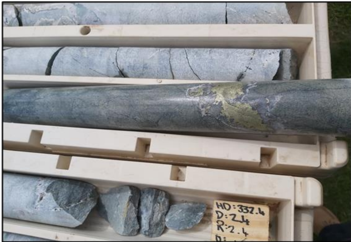
Figure 2 - Diamond Core from AWN002 from 327.2m to 331.3m showing 4.6m of quartz veining & alteration with abundant chalcopyrite stringers and disseminations (Refer to ASX announcement 'West Wyalong Drilling Intersects Potential Mineralisation').
