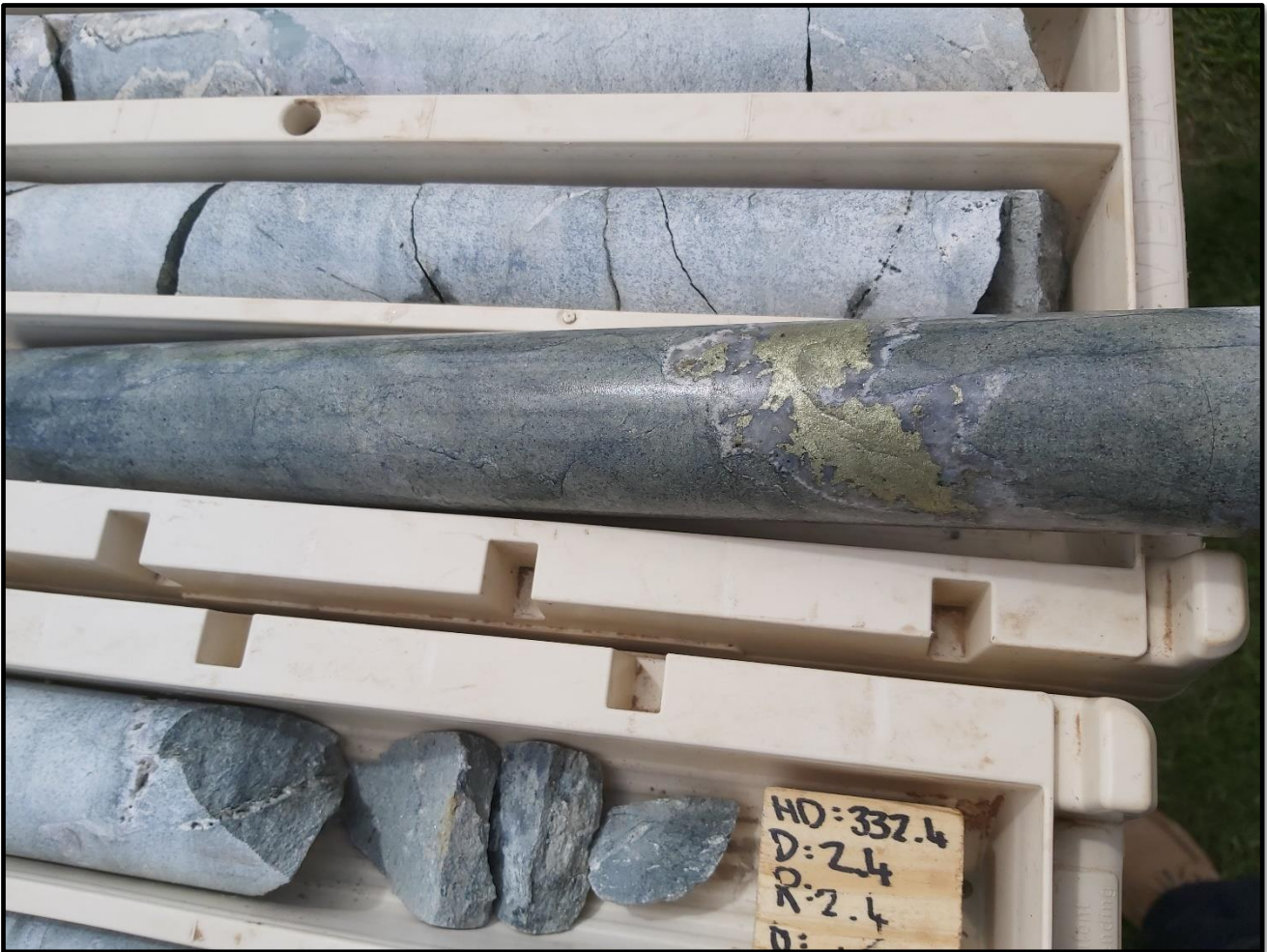
Figure 3 - Diamond Core from AWN002 from 327.2m to 331.3m showing 4.6m of massive quartz veining with abundant chalcopyrite stringers and disseminations.
