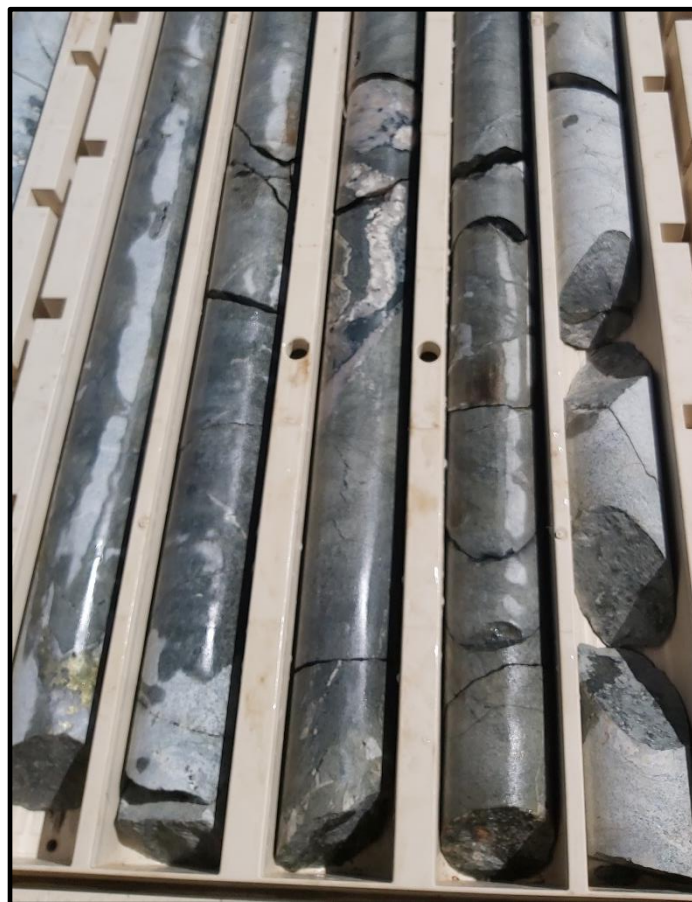
Figure 1 – AWN002 drill core with quartz veining and pyritic, chalcopyritic massive veining in chloritic-phyllitic altered host
