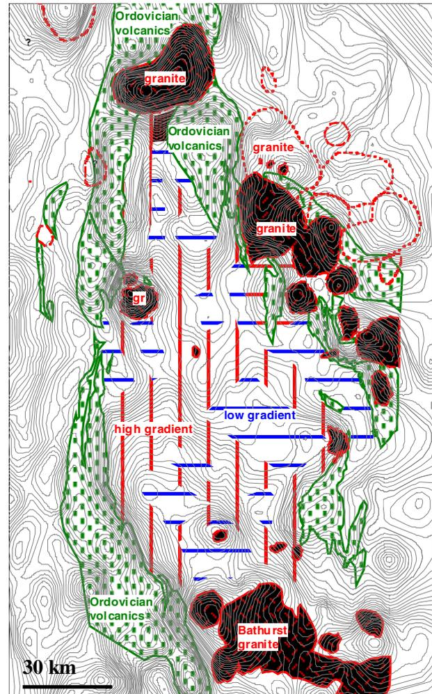
Figure 3. Subdivision of gravity contours with high gradient high (steep) zones (red vertical lines) and low gradient low (flat) zone (blue horizontal lines). Red circular features define outcropping and interpreted granites and green outlines outcropping Ordovician volcanics.
