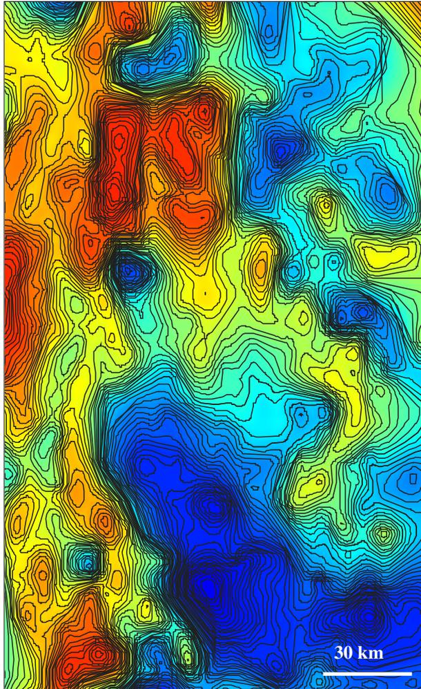
Figure 2. Regional gravity image (4 x 5 km grid) with contours above the Hill End Trough.
